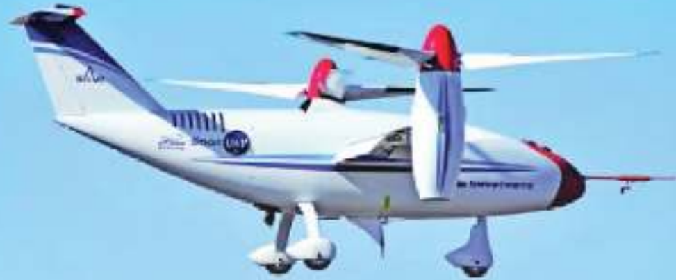
KARI is the second to develop a tiltrotor Unmanned Aerial Vehicle that takes off and lands vertically and flies at high speed.
